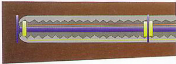
Ground anchor doubly protected
